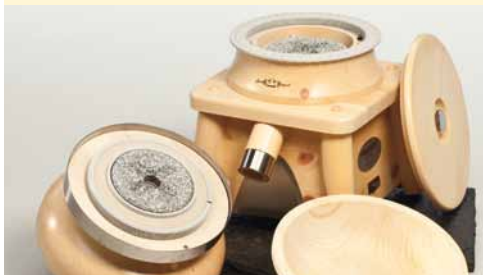
Stone grinder made of ceramic and corundum
