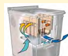
Air flow in the bio combustion chamber
